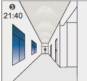
The light remains in dimming level at night.
